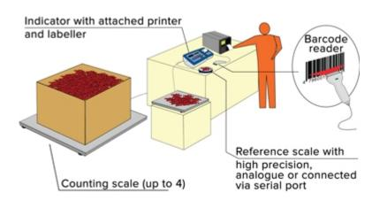
Suitable for counting applications and data management, with articles database, clients database and tares database and customisation printouts. Internal Counting Resolution up to 1.500.000 points. Up to 5 independent connectable scales. CE-M approvable (OIML R-76 / EN 45501).
