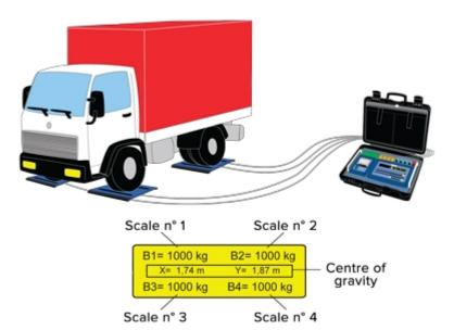
Suitable for creating wheel weighing and static axle weighing systems, or to weigh objects with various resting points. Ideal for weighing and calculating the centre of gravity coordinates of the vehicles, trucks, airplanes, containers, etc. Simultaneous display of the weight of each connected platform and of the sum. CE-M approved (OIML R-76 / EN 45501).
