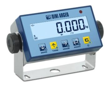
Digital weight indicator for industrial environments, easy to install and use. The IP68 protection degree and the built-in long life battery make it particularly suitable for automotive and mobile weighing applications. Standard fitted with a support bracket with adjustable inclination. CE-M approvable (OIML R-76 / EN 45501).
